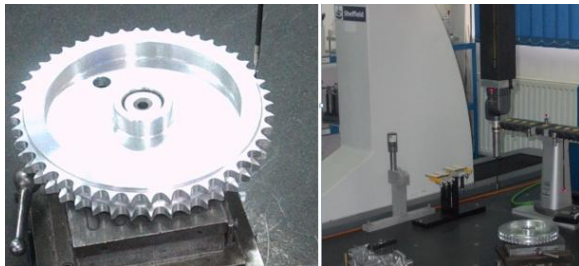
Fig. 14: Laying out sprocket on the machine table
