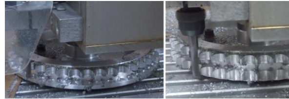
Fig. 12: Machining at to second side of tothing
