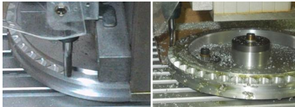
Fig. 10: Splintering evolution at first strand of the wheel tothing
