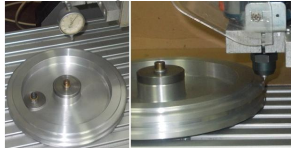
Fig. 7: Checking the work-piece position
